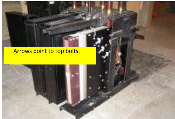
Figure 24 Top Bolts on an Arc Chute
