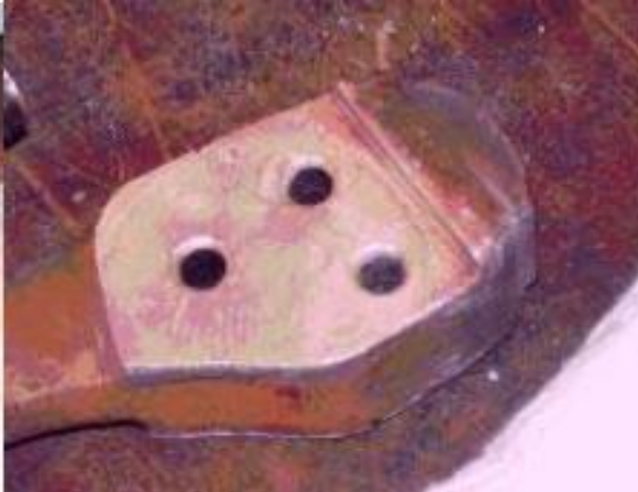
Figure 41. Silver-Plated Mating Surface
