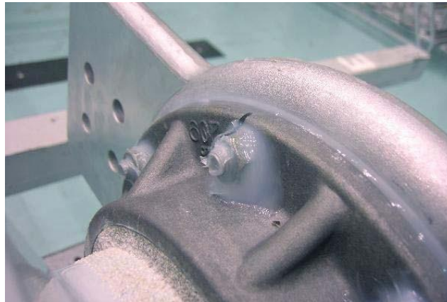
Figure 58. Correct Application of Silicone Sealant to Hardware on MEPPi Breakers
