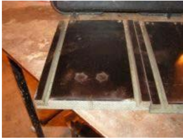
Figure 26. Bolt-Head-Shaped Deposits on Separators
