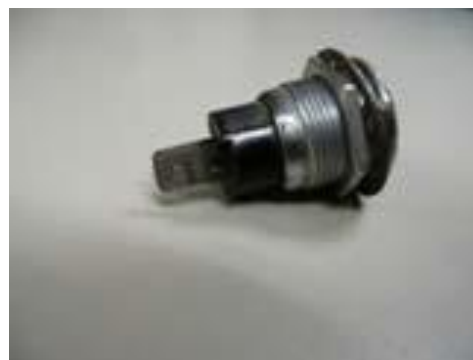
Figure 2. Receptacle Without a Resistor, Removed From the Mounting
