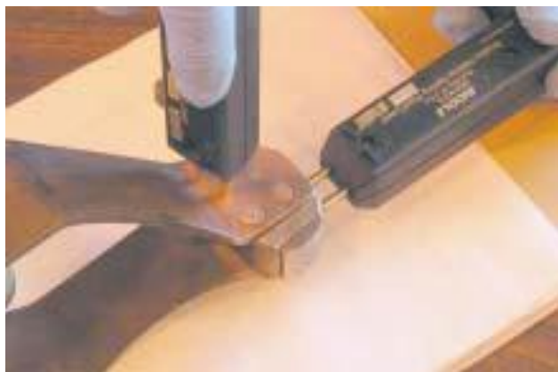
Figure 43. Testing the Contact Carrier-to-Blade Micro-Ohms
