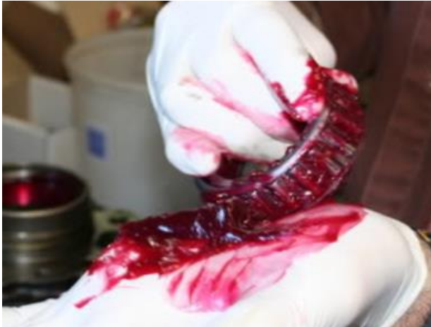
Figure 111. Technique for Packing Grease Into Roller Bearing
