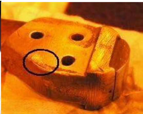
Figure 39. High Spot Removed
