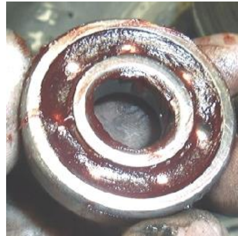
Figure 112. Fully Packed Open Ball Bearing
