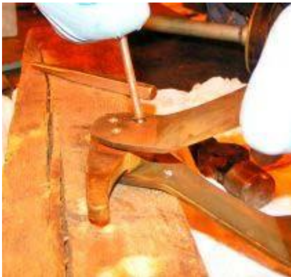
Figure 36. Breaking Off the Rivet Head
