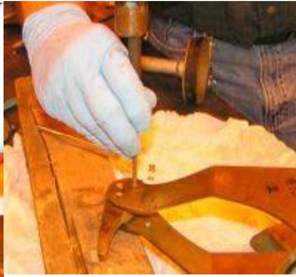
Figure 37. Driving Out the Rivet
