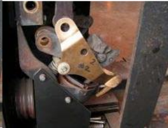
Figure 30. Hinge Pin and Spacers Removed
